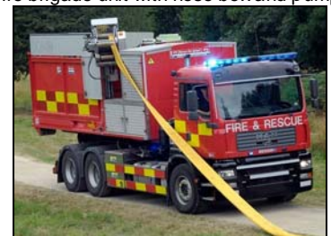
Fire brigade unit with hose box and pump
